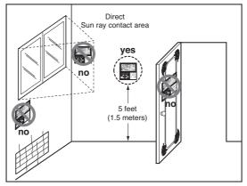
Fig.1 Typical locations for remote controller
