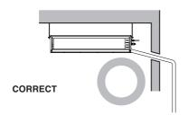
Install the P-Trap (or U-Trap) to prevent a water leakage caused by the blocking of intake air filter. Lay the drain hose with a downward inclination so water will drain out.
