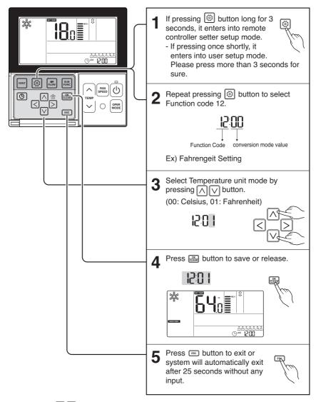
₩ Whenever press button in Fahrenheit mode, the temperature will increase/drop 2 degrees.
