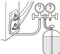
**4** Charge the refrigerant by adjusting the low-pressure valve of the manifold gauge.
