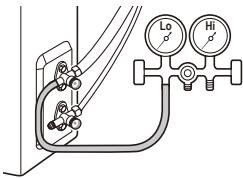
**2** Open both the gas service valve and the liquid service valve of the outdoor unit.
