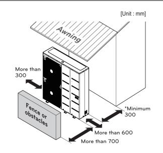
\* Please secure the space, considering field installation of the shut-off valve and strainer.
